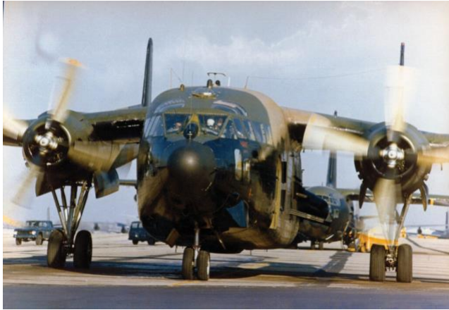
A Fairchild AC-119K Stinger stands ready for action in Vietnam. The high-powered guns of the AC-119K and AC-119G Shadow, both modified Fairchild C-119 “Flying Boxcar” cargo airplanes, provided potent ground support for U.S. troops in war zones. (San Diego Air and Space Museum)
