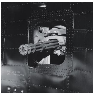
Both the AC-119G Shadow and AC-119K Stinger featured four 7.62mm rotary miniguns, though the later Stinger also boasted two 20mm M61 cannons. (U.S. Air Force)
