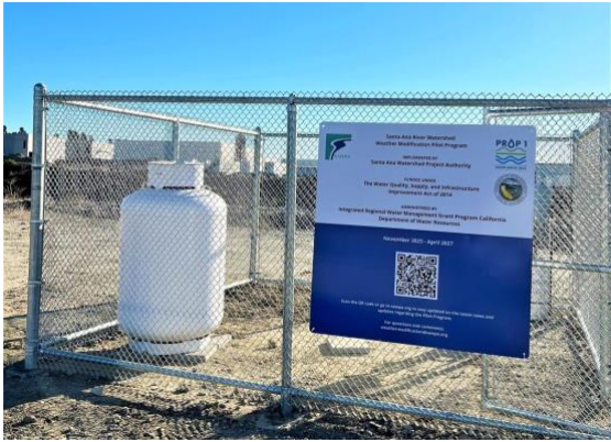
A ground-based seeding system mixes silver iodide particles and acetone, which is vaporized and released into the atmosphere. (Courtesy of SAWPA)
