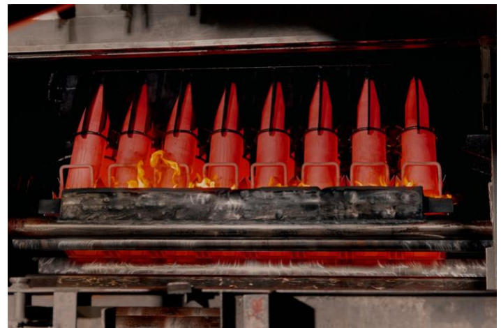
Artillery shells stand over an oil “bath” that’s designed to cool them before the final stages of assembly.
