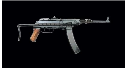
North Vietnam's home-manufactured K-50M incorporated selected components from the Soviet PPSH-41 and the French MAT-49 submachine guns. (Greg Proch)
