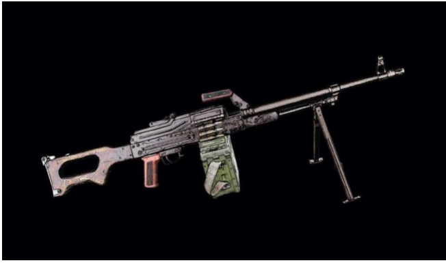
A latecomer to the war, the Soviet PK machine gun was essentially a squad machine gun based on the AK-47. Like the American M60's barrel, the PK's barrel could be changed when it overheated. (Greg Proch)
