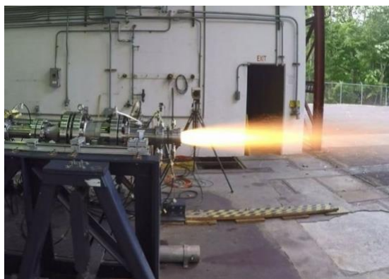
Test of Northrop Grumman's ramjet engine for extended-range 155 mm artillery shells
