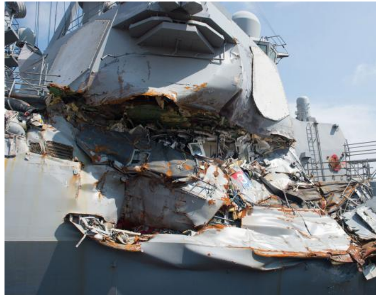
The Arleigh Burke-class guided-missile destroyer USS Fitzgerald sits in Dry Dock 4 at Fleet Activities Yokosuka to continue repairs and assess damage sustained from its June 17, 2017 collision with a merchant vessel. (U.S. Navy photo/Christian Senyk) Stars and Stripes 20 Jun 2018 By Dianna Cahn
